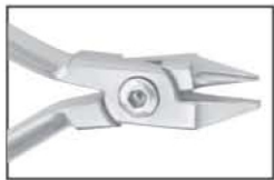
AI-1953 Bird beak plier for bending round, square and rectangle wire up to .30"/.76mm.
